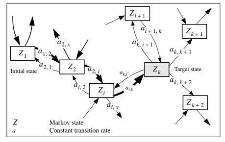
Figure 4: Part of a Markov Process with Probable (Direct) Transitions from the Initial State to the Target State Z<sub>k</sub>
