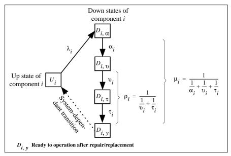
Figure 2: General Model of Components (excluding controllers)
