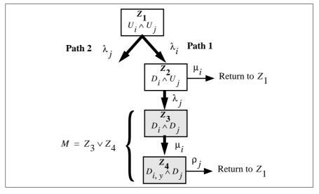
Figure 5: Modelling of the Minimal Cut Type:  $M = D_i \wedge D_j$ Markovian minimal cut model for minimal cut type  $D_i \wedge [D_C \rightarrow S_{CB}]$  [Fig. 6]
