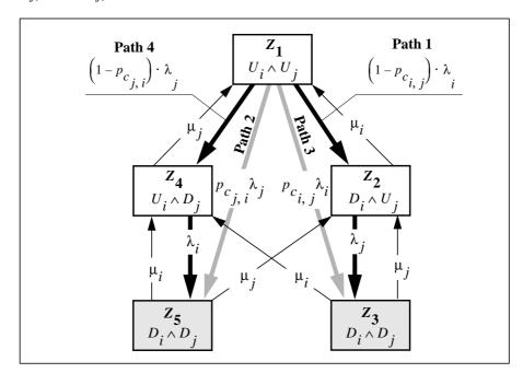
Figure 8: Modelling of the Minimal Cut Type 2. Order:  $D_i \wedge D_j$  (Markov Minimal Cut Model 2. Order)
