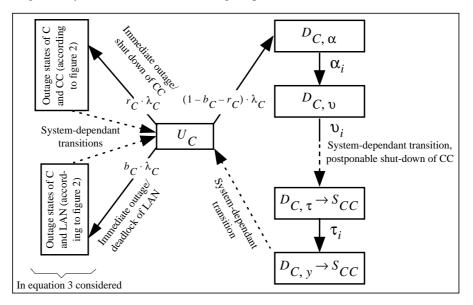
Figure 3: Component Model of a Controller with Influence/Dependencies to other Components
