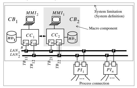
Figure 1: Central Automation and Control System
