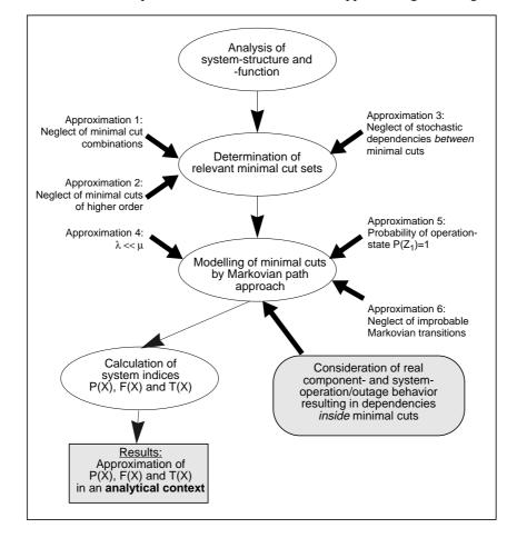
Figure 7: Overview on Markovian Minimal Cut Approach with Approximation Steps
