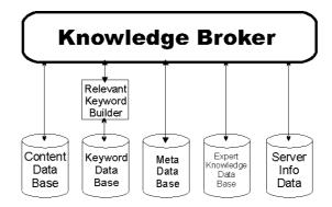
Figure 2: Architecture of the Information Broker System
