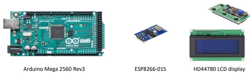
Figure 6: Hardware components: ATmega2560, ESP8266 and LCD display
