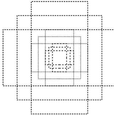
Figure 4: *Faster-RCNN anchors. In this example the network is configured to use 9 anchors (3 bounding boxes in 3 scales denoted by different line styles)*
