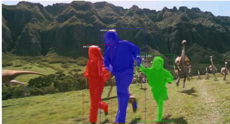
Figure 3: *Mask-RCNN*, aside from performing object detection, effectively differentiates between objects and the background, even if the image quality is imperfect
