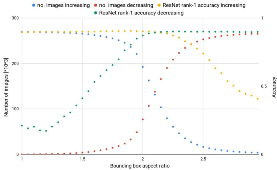
Figure 9: The chart visualising the bounding box aspect ratio thresholds influence on the number of images and re-identification accuracy
