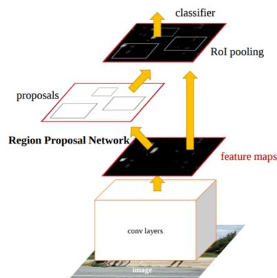
Figure 5: *Faster-RCNN general architecture. Image source: [Ren et al., 2017]*
