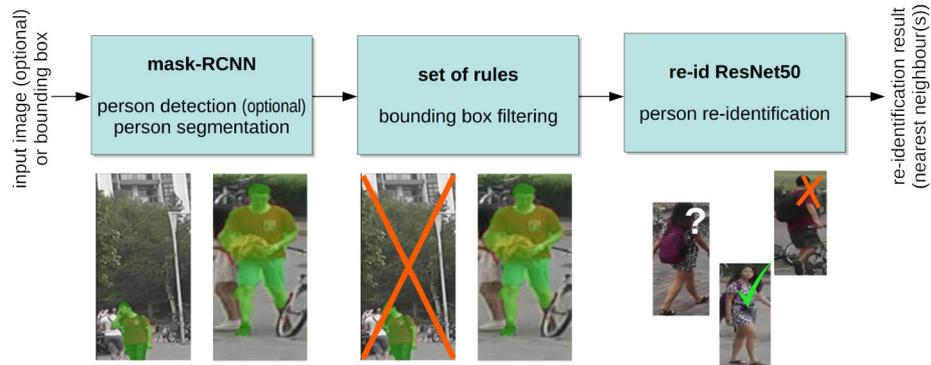
Figure 7: The flow of data across the functional blocks in the processing pipeline
