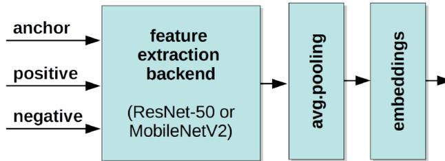
Figure 2: Block diagram of re-identification neural network architecture. The 'positive' and 'negative' inputs are used only during the training phase
