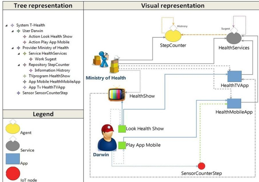
Figure 7: Architecture of cross-device tests with mobile and Digital-TV
