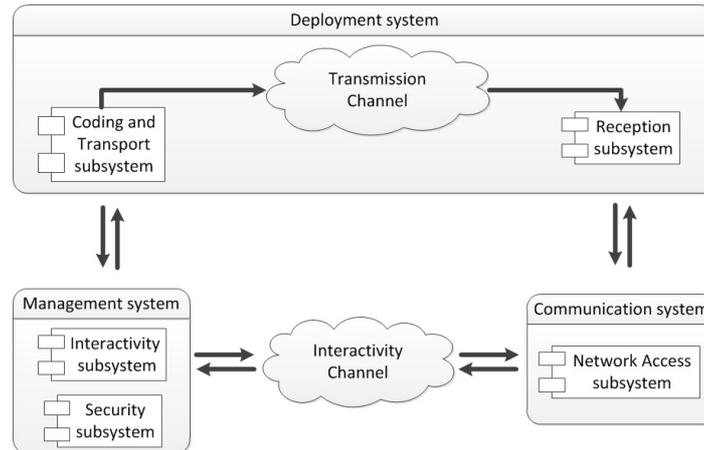
Figure 4: Interaction of the subsystems of the architecture
