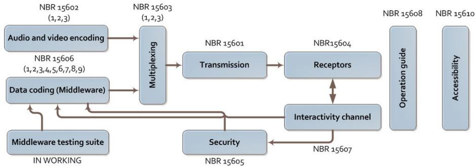
Figure 1: Technical standards for the digital TV ISDB-T standard [ABNT 2004]
