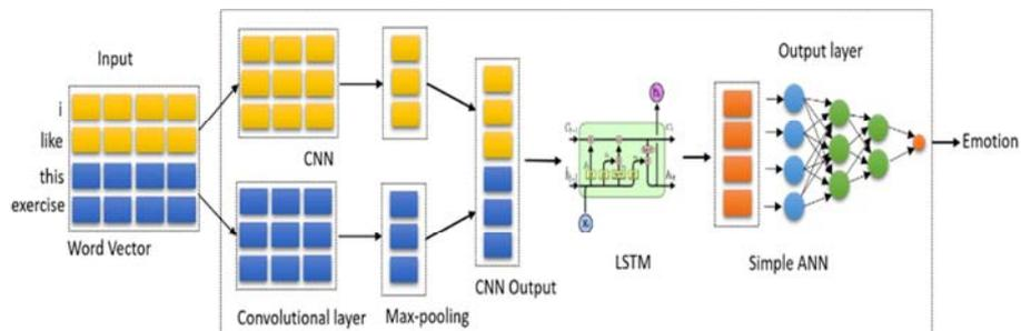
Figure 2: Model 6: DL with CNN and LSTM.
