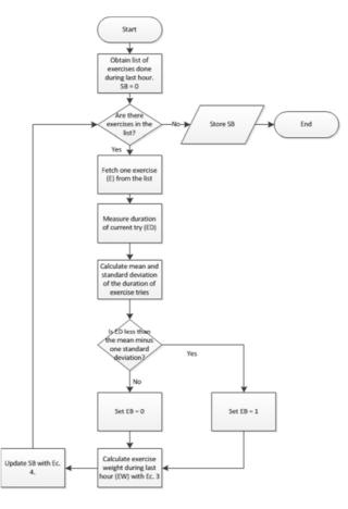
Figure 4: Flow of rules for the detection of boredom
