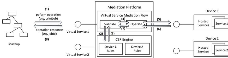
Figure 6: Detecting and Blocking Invalid Invocations
