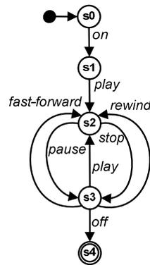
Figure 3: FSM for Complex Behaviour of the Service Video Streaming hosted in Device Vide
