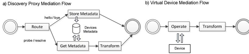
Figure 5: Discovery Proxy and Virtual Devices' Mediation Flow
