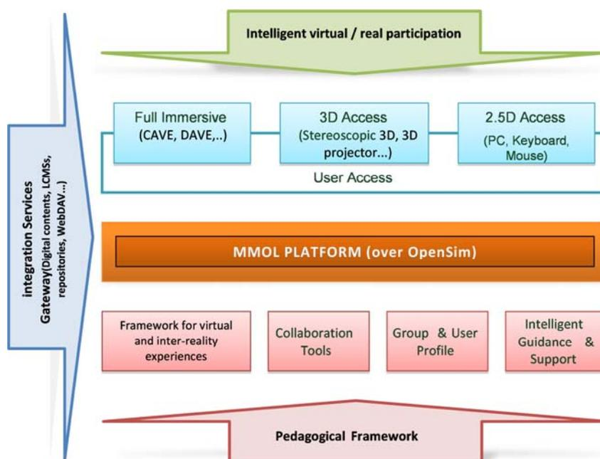
Figure 1: SLRoute server architecture (Adapted from [Lorenzo, 2012])
