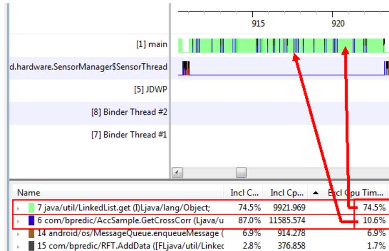
Figure 14: Mobile application profiling results showing functions which are main contributors to CPU load
