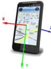
Figure 1: Acceleration sensor axis on testbed mobile device
