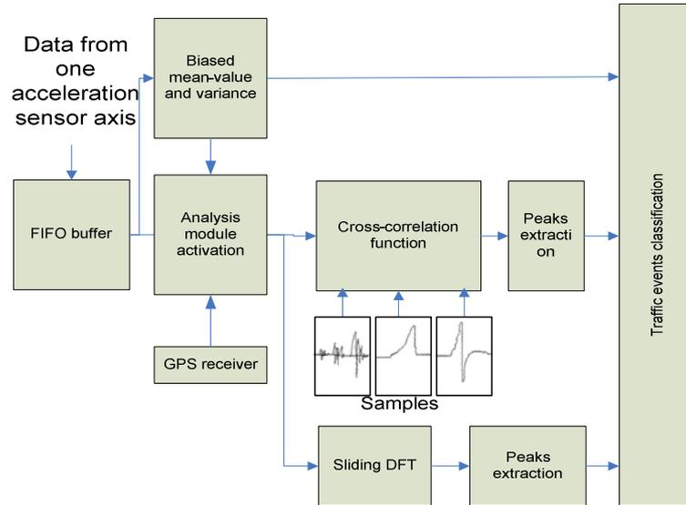
Figure 6: Accelerometer data flow during analysis
