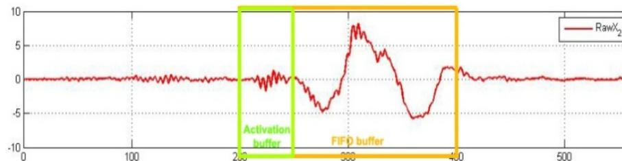
Figure 5: FIFO buffer used for accelerometer data analysis
