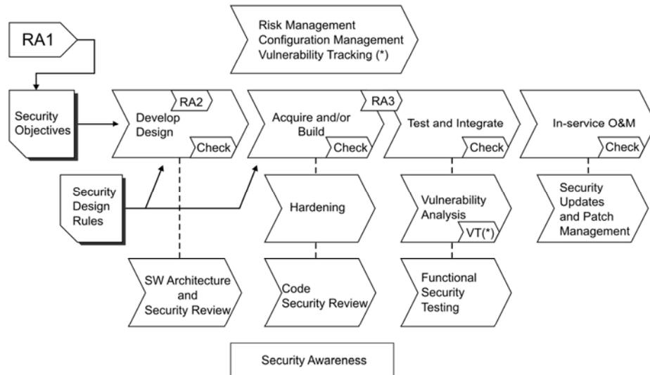
Figure 5: Illustration of Ericsson's RA process in Waterfall SW development.
