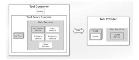
Figure 1: Simplification of LTI architecture: BLTI architecture (in gray)
