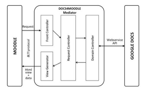
Figure 9: Technical Architecture of Mediator
