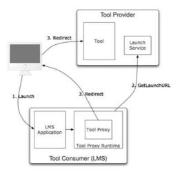
Figure 2: BLTI Launch process diagram.
