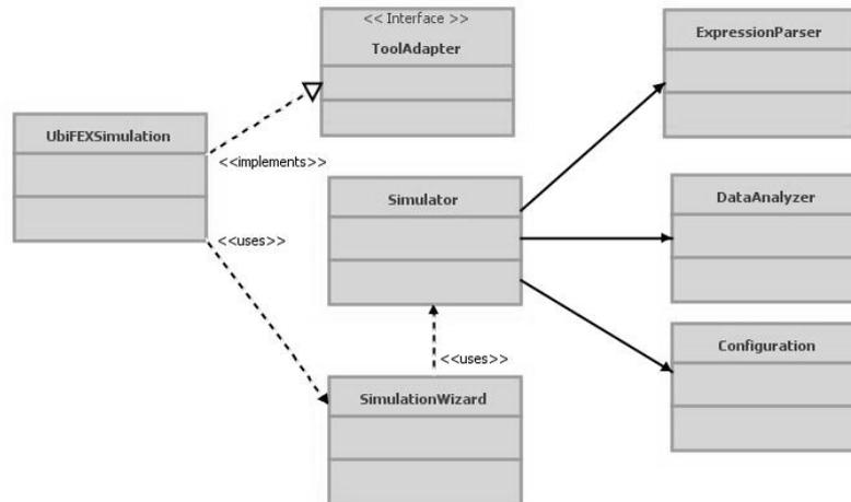
Figure 11: UbiFEX Simulation – Simplified class diagram
