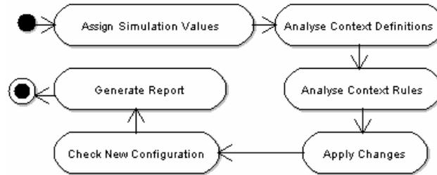
Figure 8: Steps of the verification process
