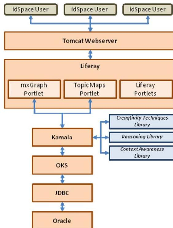
Figure 1: Top level Architecture of IdSpace platform
