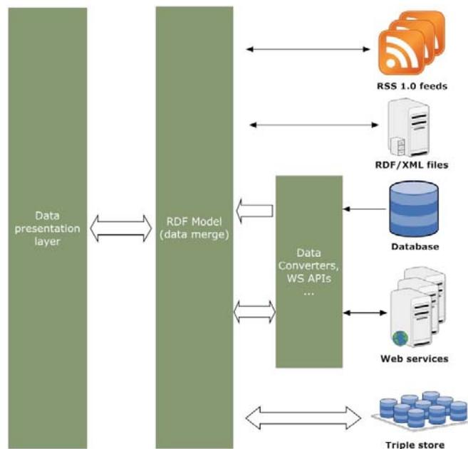
Figure 9: Sweb high-level architecture
