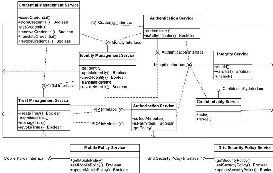
Figure 3: Services and interfaces of Security Architecture instantiated for this case study
