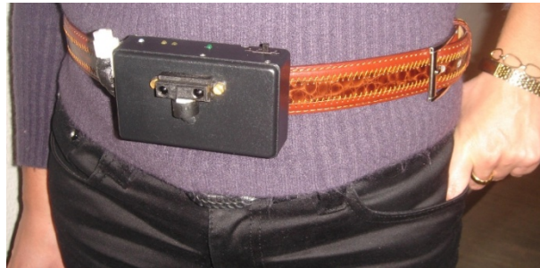
Figure 5: The prototype of our module that detects both user orientation and obstacle distance
