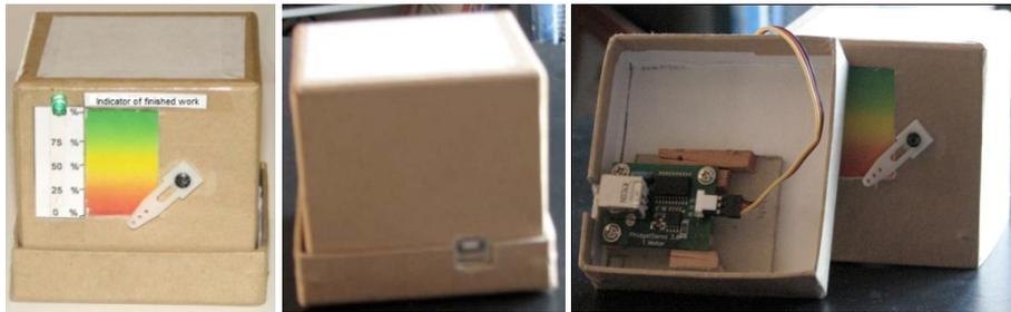
Figure 3: *Prototype of the Augmented Object, which use an USB port*
