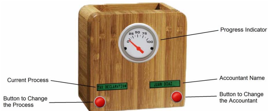
Figure 4: *Augmented pencil holder designed for the client*
