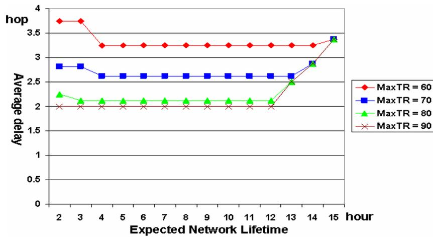
Figure 10: Average end-to-end transmission delay VS. Expected network lifetime
