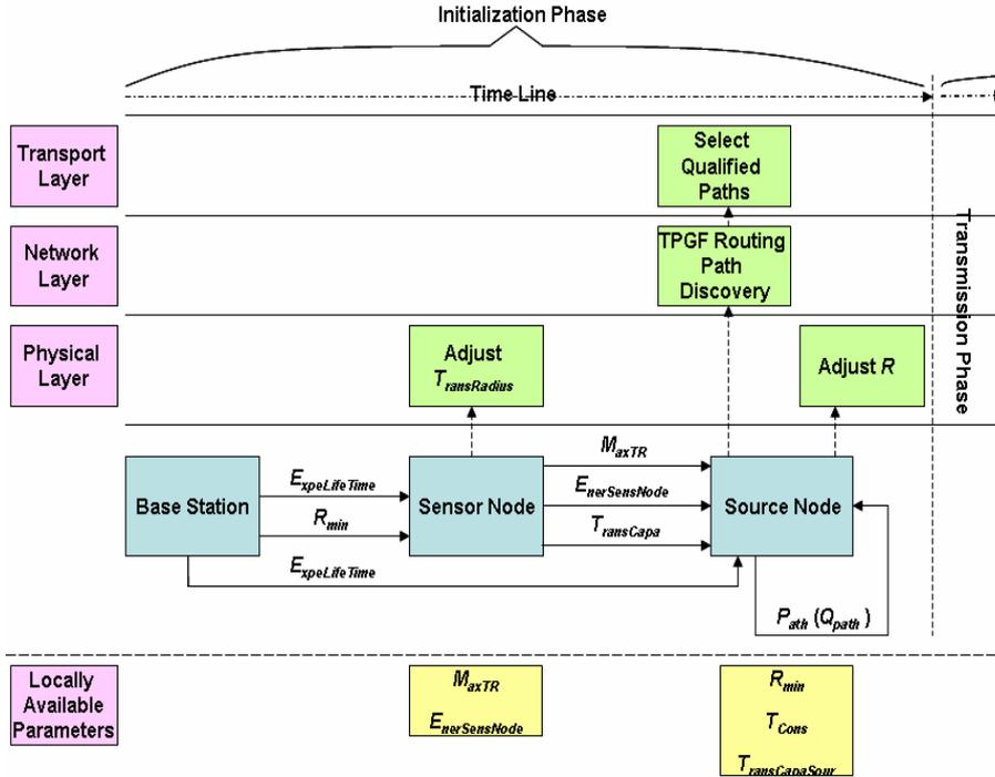
Figure 1: The cross layer framework of RRA scheme
