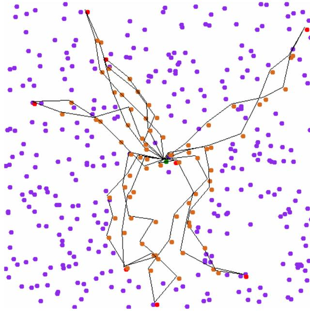
Figure 6: The simulated sensor network ( $M_{axTR} = 60 M$ ): every source node can use at least two paths. The number of transmission hops of each routing path is smaller than 12. The location of the base station is randomly chosen, where the number of neighbor nodes of the base station is limited.
