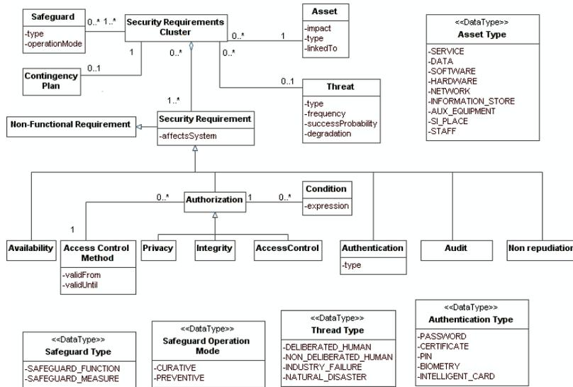
Figure 3: Extending the metamodel of Fig. 2: general security concepts
