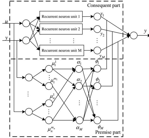
Figure 2: Schematic scheme of RFNN
