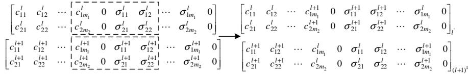
**Figure 3:** Schematic scheme of the crossover operation
