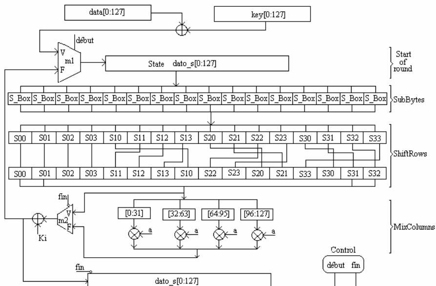
Figure 4: Diagram for the Cipher module
