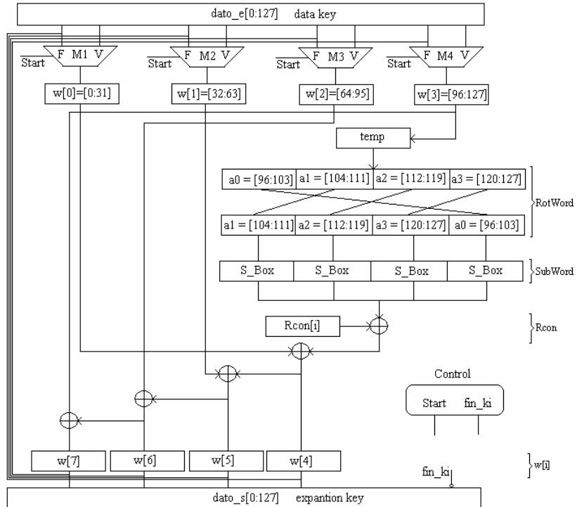
Figure 3: Diagram for the Expansion\_ki module for only one round
