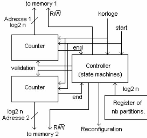
Figure 5: Diagram of the controller
