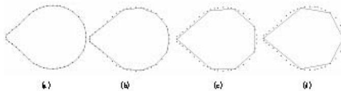
Figure 5: The approximate result using variational acceleration factor and fitness function. (a) Original curve, where  $n = 46$ . (b) The first approximate result, where  $m = 11$ ,  $c_4 = 1$ ,  $c_5 = 0$ ,  $c_6 = 110$ ,  $e = 8.45$ . (c) The second approximate result, where  $m = 7$ ,  $c_4 = 1$ ,  $c_5 = 0$ ,  $c_6 = 70$ ,  $e = 36.3$ . (d) The third approximate result, where  $m = 6$ ,  $c_4 = 1$ ,  $c_5 = 0$ ,  $c_6 = 60$ ,  $e = 82.4$ .
