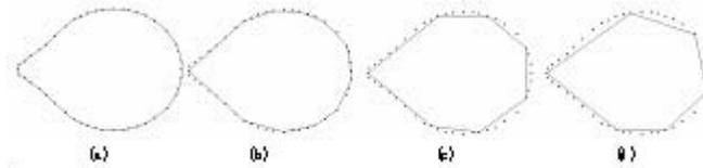
Figure 6: The approximate result only using variational acceleration factor. (a) Original curve, where  $n = 46$ . (b) The first approximate result, where  $m = 11$ ,  $c_4 = 1$ ,  $c_5 = 0$ ,  $c_6 = 0$ ,  $e = 8.4$ . (c) The second approximate result, where  $m = 7$ ,  $c_4 = 1$ ,  $c_5 = 0$ ,  $c_6 = 0$ ,  $e = 37.0$ . (d) The third approximate result, where  $m = 6$ ,  $c_4 = 1$ ,  $c_5 = 0$ ,  $c_6 = 60$ ,  $e = 87.8$ .
