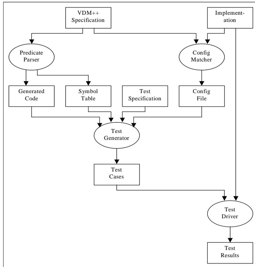
Figure 1: Architecture of the TESTAF
