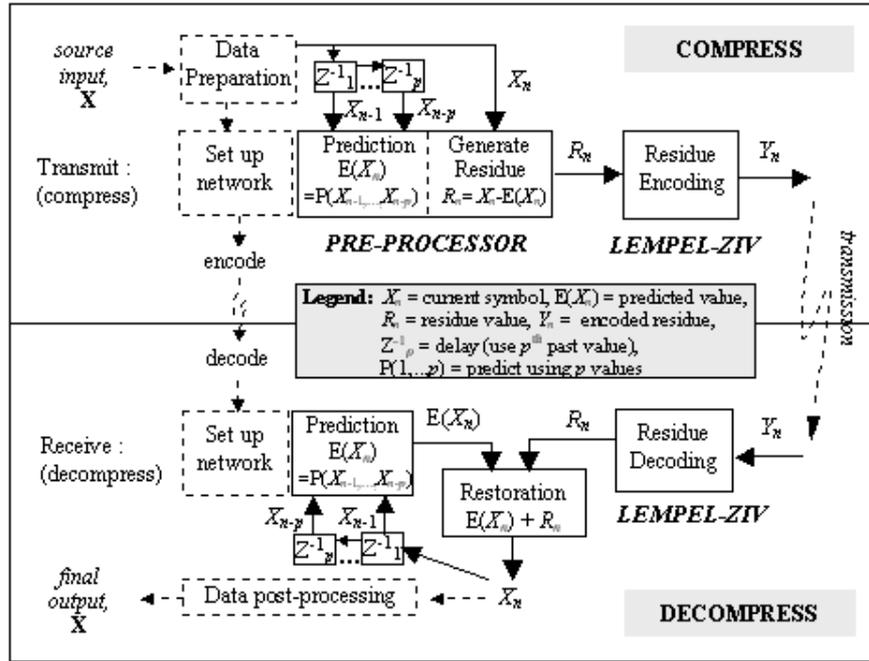
Figure 3: Implementation schematic of the two-stage scheme
