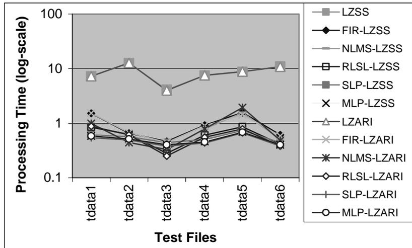
Figure 5: Processing time achieved by the encoder-only and two-stage schemes for the different test files
