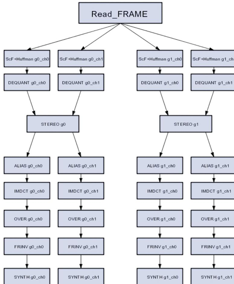
**Figure 5:** Screen shot of the task graph of the MP3 decoder.
