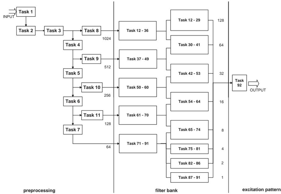
Figure 6: Task graph of the simulator of the human peripheral auditory system. The task required for sampling is not depicted in this figure.
