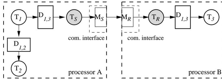
Figure 3: Realizing buffered intra- and inter-processor communication by introducing buffers ( $D_{ij}$ ) and communication tasks ( $T_S$  and  $T_R$ ). Inter-processor communication is realized by point-to-point links with hardware buffers of limited size ( $M_S$  and  $M_R$ ) and may result in the synchronization of  $T_S$  and  $T_R$ .
