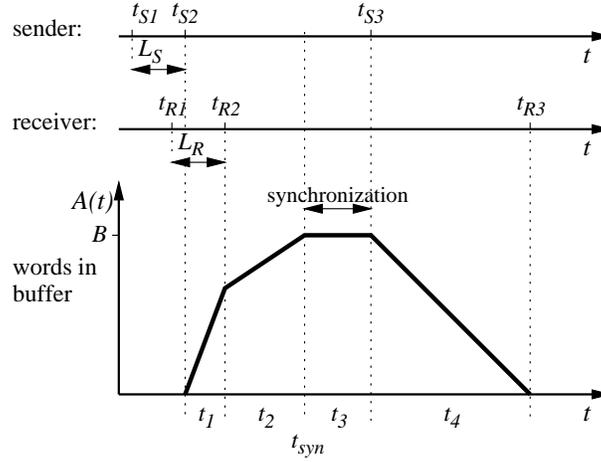
**Figure 4:** Timing diagram of a synchronized inter-processor communication.
