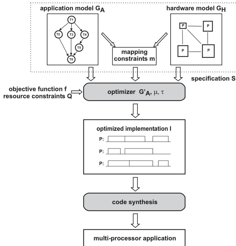
Figure 1: Overview of our prototyping framework PEPSY. PEPSY approximates an optimal implementation  $I$  given a specification  $S$  (consisting of an application model, a hardware model and mapping constraints) subject to an objective function and resource constraints. The optimizer extends the application model by introducing communication tasks and computes a mapping  $\mu$  and schedule  $\tau$ . The optimized implementation is then automatically synthesized.
