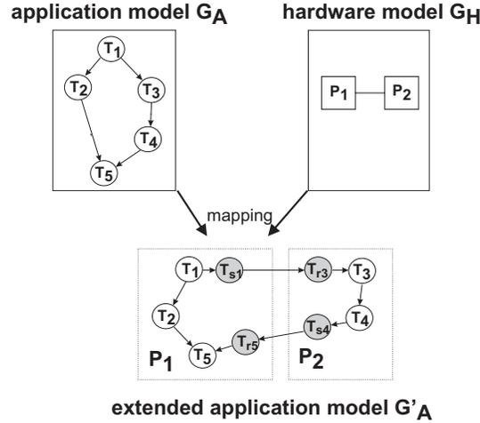
Figure 2: Extended application model  $G'_A$ . Every arc between tasks mapped onto different processing elements is replaced by a pair of communication tasks.
