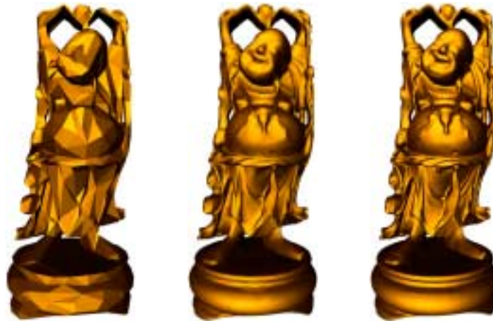
Figure 1: Progressive transmission of a complex 3D object (the Stanford Buddha) created from multiple 3D scans. Initial representation with 3,774 triangles (left), intermediary representation with 30,392 triangles (middle), complete mesh consisting of 1,087,716 triangles (right). (courtesy L. Kobbelt, R. Schneider, H-P. Seidel; RWTH Aachen and MPI Saarbrücken)
