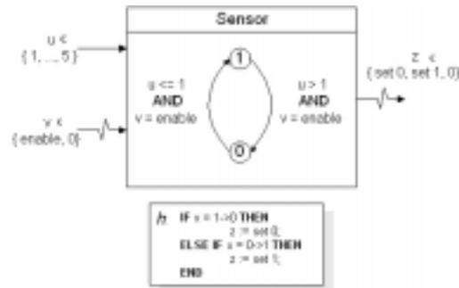
Figure 5: Sensor module
