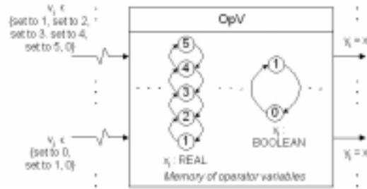
Figure 4: The OpV module
