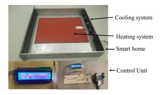
Figure 8: The appearance of the Smart Home simulator
