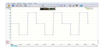
Figure 10: The graph of ambient temperature set-point
