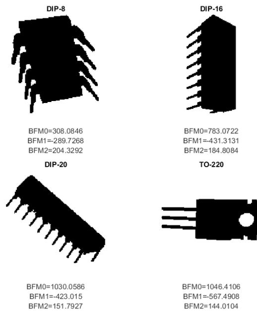
Figure 5: Illustration of Bessel-Fourier moments obtained for various sample IC packages
