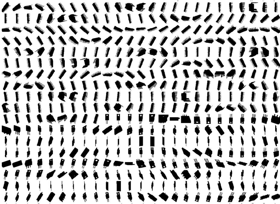
Figure 1: Sample binary images captured for various views of exemplary IC packages
