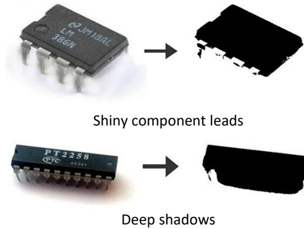
Figure 3: Illustration of some problems caused by illumination influencing the binarization results
