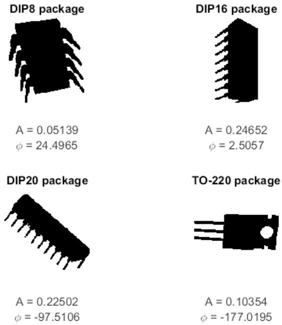
Figure 6: Illustration of Zernike moments obtained for various sample IC packages
