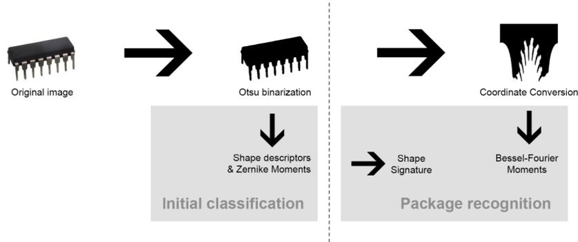
**Figure 8:** The simplified flowchart of the proposed method
