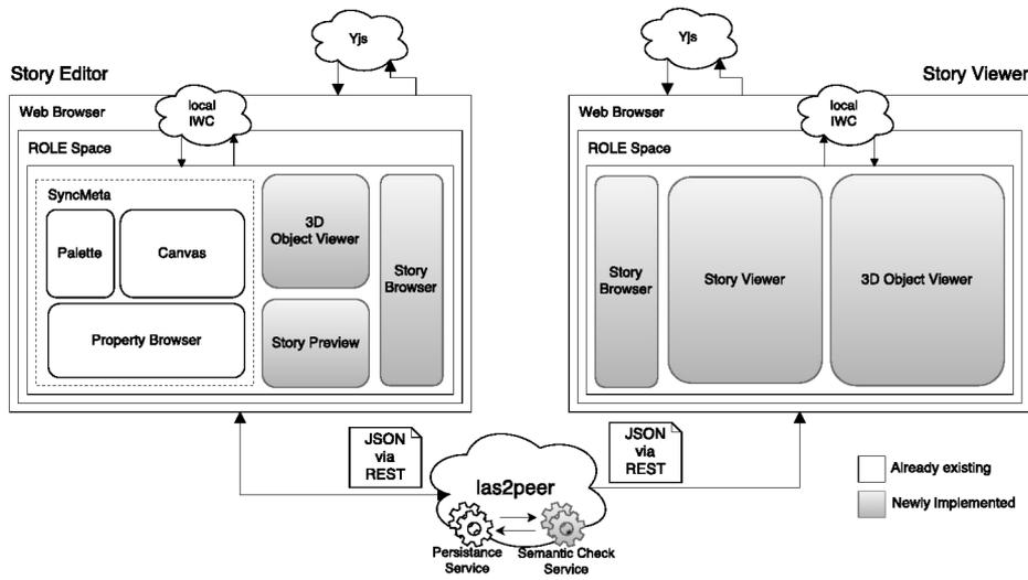
Figure 5: Architecture diagram. Note, that the widgets to be created in the story editor are congruent to the ones in the story viewer.
