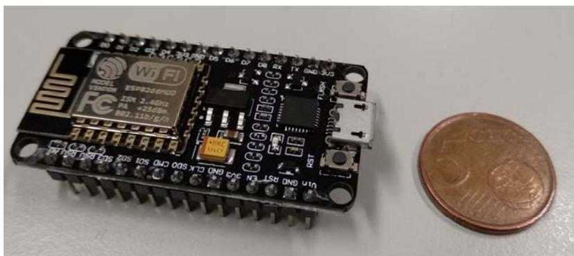
Figure 2: A second generation ESP8266 ESP-12E NodeMCU Amica board.
