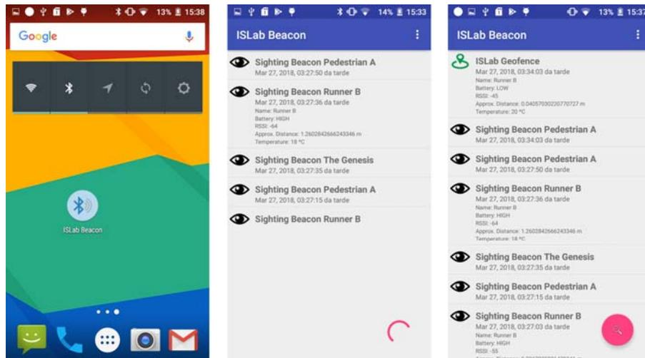
Figure 9: Android's ISLab Beacon app. From the left to the right: (1) app's launcher icon; (2) scanning for nearby Smart Clothing; (3) details of two Runner B sightings.
