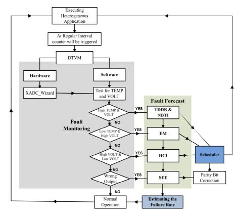
application is stored in the memory. The SEU processes will be carried out so that bit flip will be corrected.
