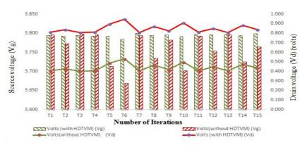
Figure 7: Voltage variation with and without DTVM
