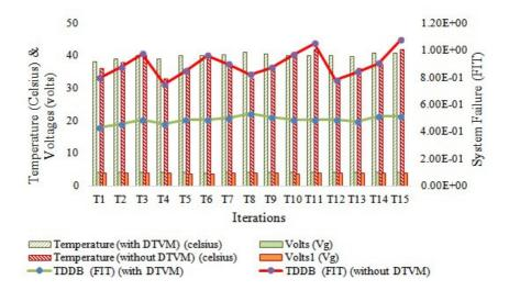
Figure 8: Failure rate for the TDDB with and without DTVM
