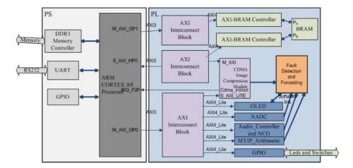
Figure 4: Complete infrastructural design in Zedboard.
