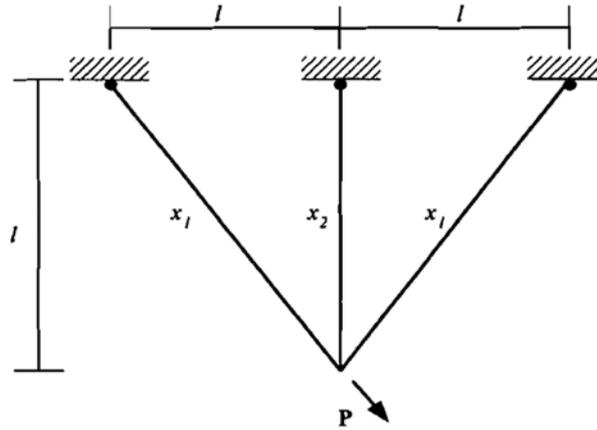
Figure 4: Three-bar truss design problem
