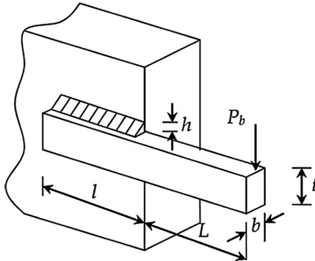
Figure 3: Welded beam design problem
