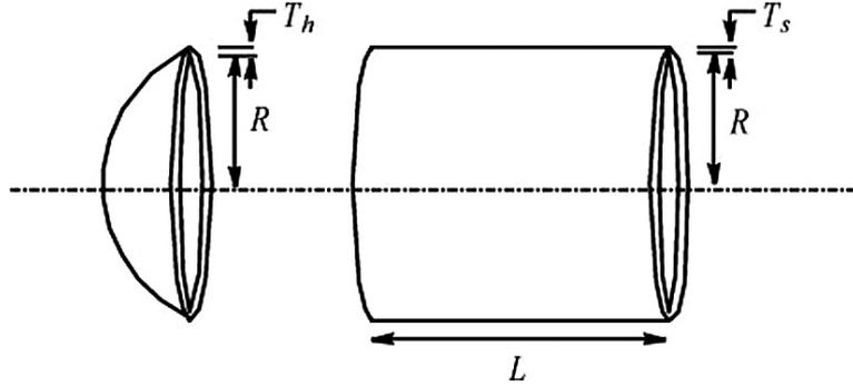
Figure 5: Pressure vessel design problem
