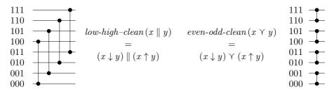
Notice that the two cleaners are in a sense dual to each other: numbering the inputs in binary (most significant digit first), the low-high cleaner connects inputs 0w and 1w, while the even-odd cleaner connects inputs w0 and w1.
