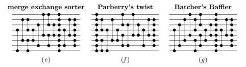
The altered layout of (g) compared to (e) reflects the iterative nature of these presentations. Algebraically, it can be computed by unfolding the recursion then rearranging the components using the interchange law (16d), so for example:
