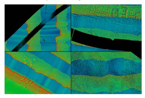
Figure 7: Point density maps of LiDAR datasets 1, 2, 3, and 4
