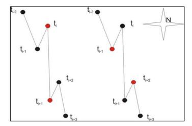
Figure 3: Proximity correction of void border points
