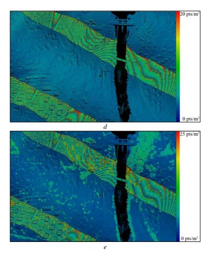
Figure 8: LiDAR point density maps of individual strips (a-c) and strip overlapping (d and e)
