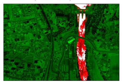
Figure 2: LiDAR points bordering on voids (red)
