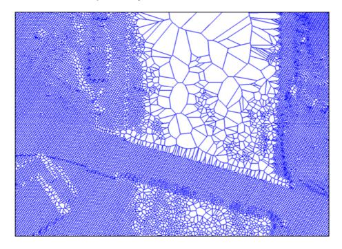
Figure 4: Voronoi diagram of LiDAR points from a region of the dataset displayed in figure 2
