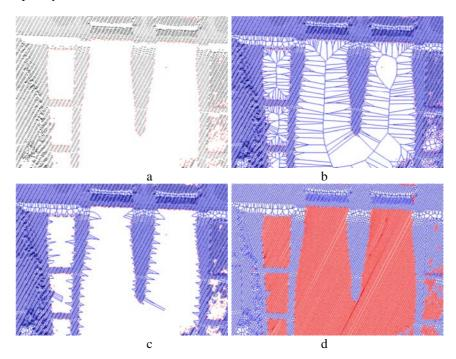
Figure 6: LiDAR weak return void borders (a), Voronoi diagram of the LiDAR dataset (b), Voronoi diagram with culled void regions (c), weak return void reconstruction (d)
