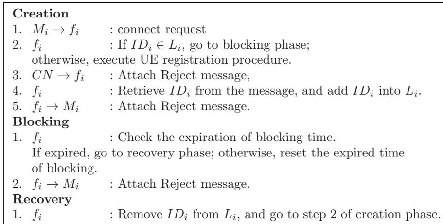
**Figure 3:** Auto-reject mechanism
