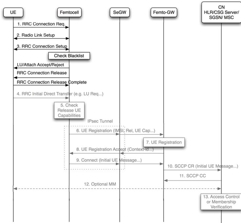
Figure 4: The benefit of auto-reject mechanism. Gray text signifies omitted steps.
