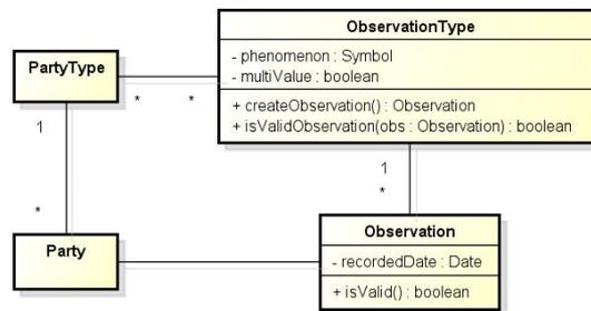
Figure 5: AOM Core Design (adapted from [Yoder et al., 2001]).
