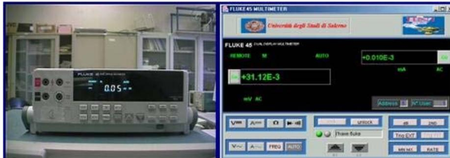
Figure 3: Real instrument and the virtual graphic interface offered to the students by Fluke45 Service
