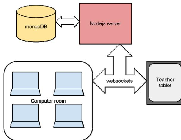
Figure 1: Scalable classON technology and architecture
