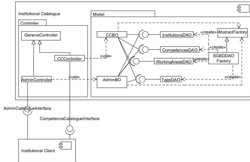
Figure 6: Competence Catalogue Component Diagram, it shows a client and an institutional catalogue, this one has a controller that switches accesses depending on the functionalities to use
