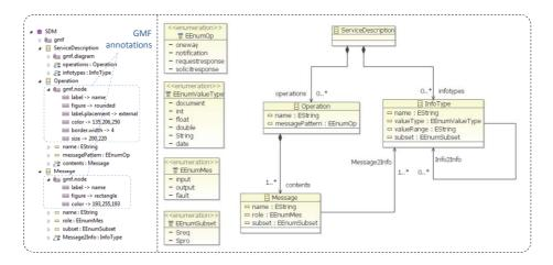
Figure 3: The ASD metamodel as an Ecore metamodel
