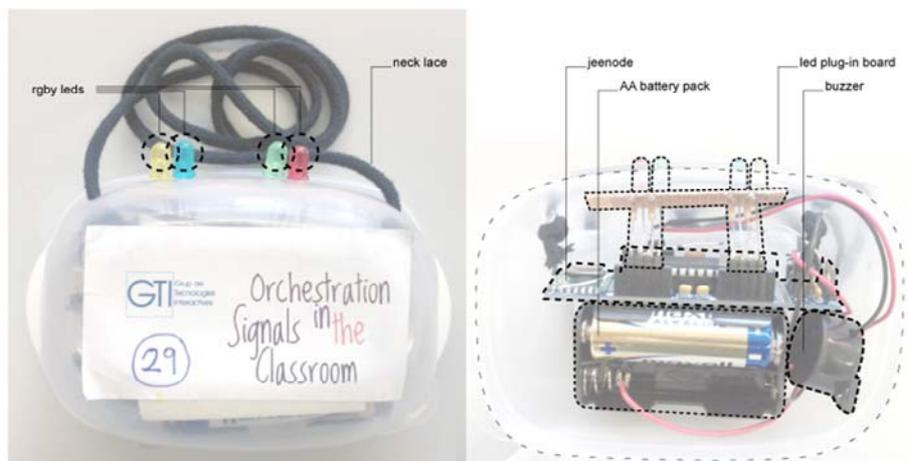
Figure 3: Necklace device: closed on the left, and open on the left. A Belt design of this device has been also built
