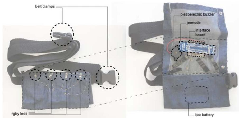
Figure 4: Textile device (as a belt): ready to be worn- on the left, unfold on the right
