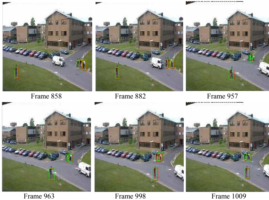
Figure 3: Image sequence one, the proposed system show the ability to track people in complex situation “The red rectangle show the location where the object detected and the green one show the predicted position by the system.”
