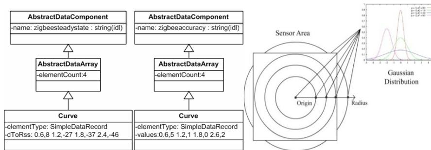
Figure 3: SensorML Description of a ZigBee Receiver Steady State Response Curve and associated Error Response Curve.
