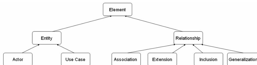
Figure 1: Meta-model of the use case diagrams domain.
