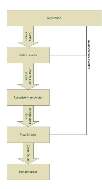
Figure 1: The pipeline of the graphics hardware (limited for the purpose of this paper)
