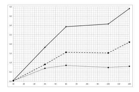
Figure 2: The (GPU time)/(CPU time) ratio for m = 15 processors. Values greater than 1 indicate that GPU implementation is faster than CPU implementation. G8 – dotted line, G32 – dashed line, G112 - solid line
