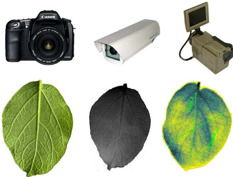
Figure 3: Instruments used in visible, near infra, and thermal infra spectral analyses of potato resistance test and images of a potato leaf taken in visible, near infra and thermal infra spectrum
