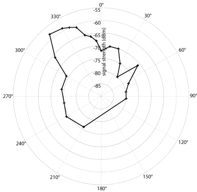
Figure 4: Vagi signal strength versus angle, June 16 2003. Target is at 330 degrees bearing (upper-left), approximately 75 feet from the antenna.
