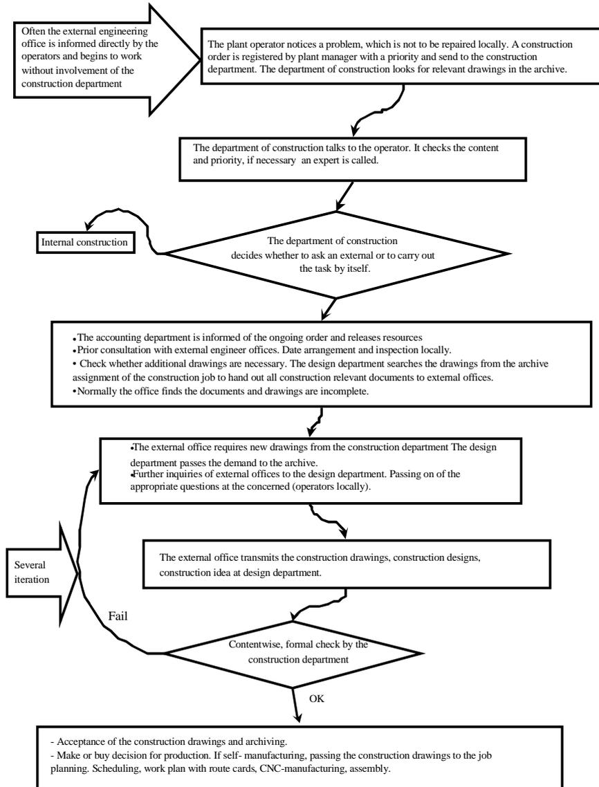
Figure 2: Typical process when constructing
